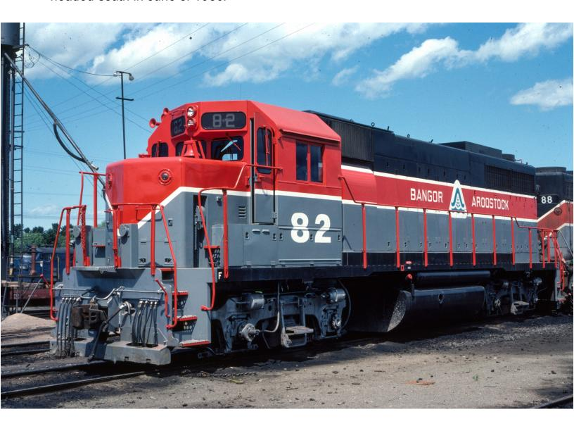
Above: David Hamley photographed 82 at NMJ on June 10, 1981 – she was painted in May of 81 into this scheme. Note the Nose bell that has been retained. 82 also has a winterization hatch over its front cooling fan (box looking affair over the forward of the two cooling fans on the rear of the long engine hood) this was the only GP38 to have this hatch.
